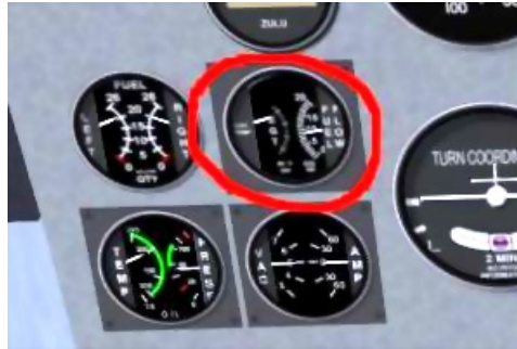
Figure 9.14: Fuel Flow and EGT gauges
