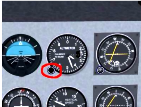
Figure 9.7: Altimeter calibration knob
