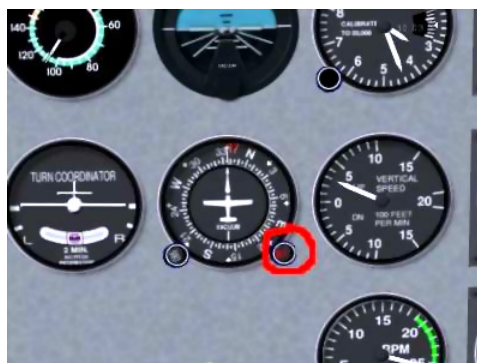
Figure 9.8: Heading adjust knob
