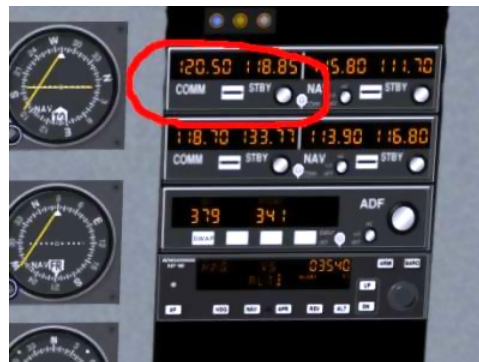
Figure 9.4: The C172 communications stack with COMM1 highlighted
