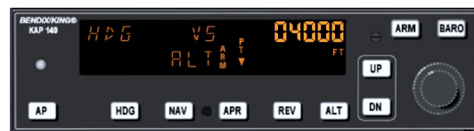
FIGURE 10.10 – Autopilot with altitude armed
