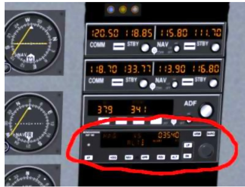
FIGURE 9.10 – The C172 Autopilot
