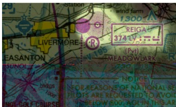
Figure 10.12: REIGA nondirectional beacon
