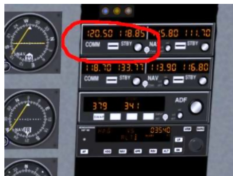
Figure 9.4: The C172 communications stack with COMM1 highlighted
