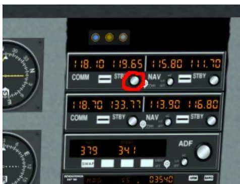
Figure 8.5: COMM1 adjustment knob
