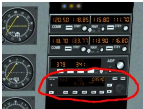
Figure 8.10: The C172 Autopilot
