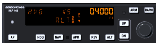
Figure 9.10: Autopilot with altitude armed
