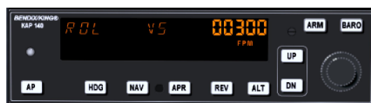
Figure 9.7: Autopilot after engaging
