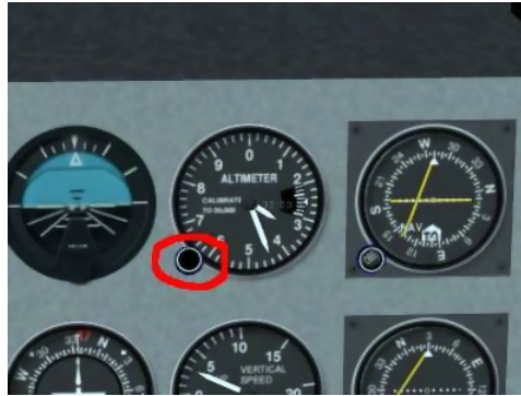
Figure 6.7: Altimeter calibration knob
