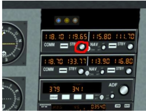
Figure 6.5: COMM1 adjustment knob
