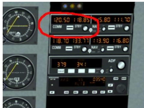
Figure 6.4: The C172 communications stack with COMM1 highlighted
