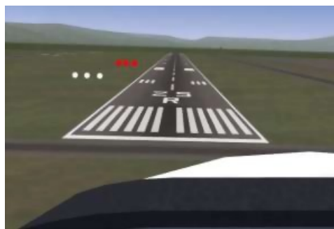
FIGURE 9.17 – On Final at Livermore with VASI on the left
