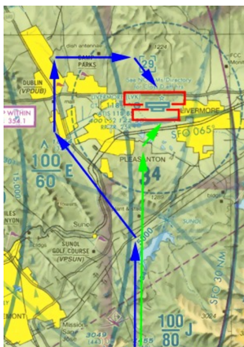
FIGURE 9.16 – Sectional extract showing approaches to Livermore
