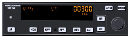
Figura 10.6: Autopilot after engaging
