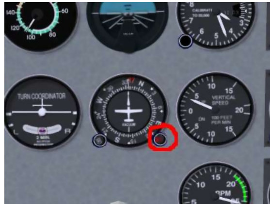
Figura 9.8: Heading adjust knob
