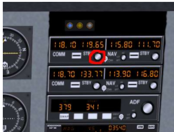
Figura 9.5: COMM1 adjustment knob
