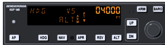
Figura 10.9: Autopilot with altitude armed
