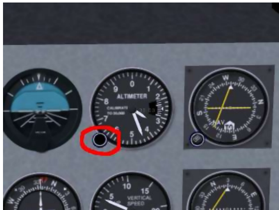
Figura 9.7: Altimeter calibration knob
