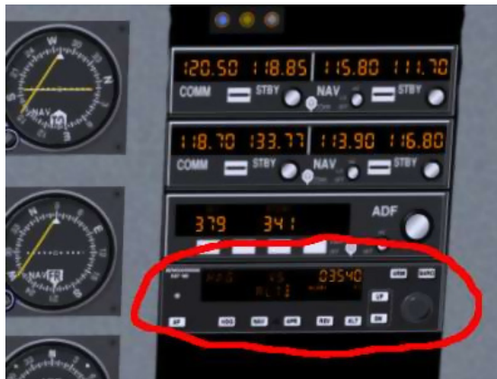
Figure 9.10: The C172 Autopilot
