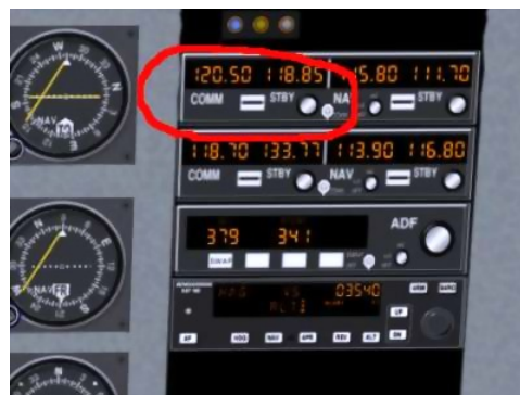
FIGURE 9.4 – The C172 communications stack with COMM1 highlighted
