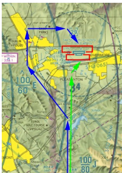
FIGURE 9.16 – Sectional extract showing approaches to Livermore
