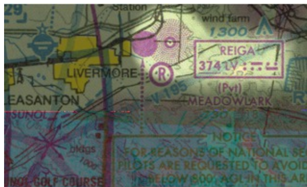
FIGURE 10.13 – REIGA nondirectional beacon
