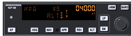
FIGURE 10.10 – Autopilot with altitude armed
