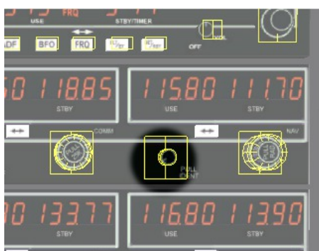
FIGURE 10.6 – Ident volume knob and hot-spots
