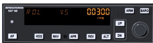
FIGURE 10.7 – Autopilot after engaging
