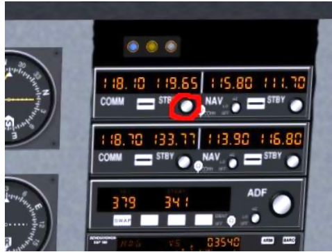
FIGURE 9.5 – COMM1 adjustment knob
