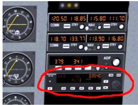
FIGURE 9.10 – The C172 Autopilot
