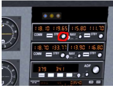
Figure 9.5: COMM1 adjustment knob
