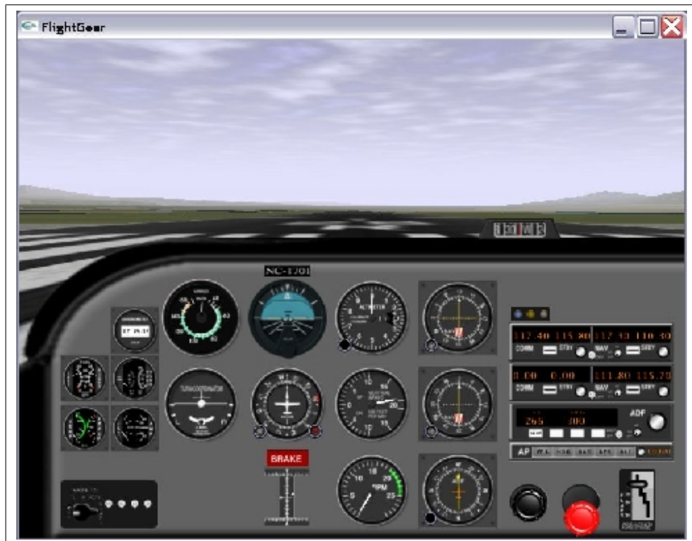
Fig. 5: The Cessna 172p 2-D instrument panel.
