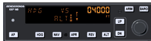
FIGURE 10.9 – Autopilot with altitude armed
