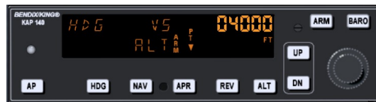
FIGURE 10.9 – Autopilot with altitude armed
