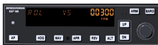
Figure 10.7: Autopilot after engaging
