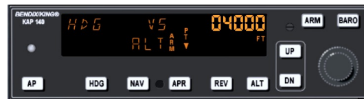
Figure 10.10: Autopilot with altitude armed
