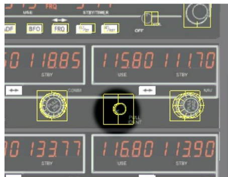
Figure 10.6: Ident volume knob and hot-spots
