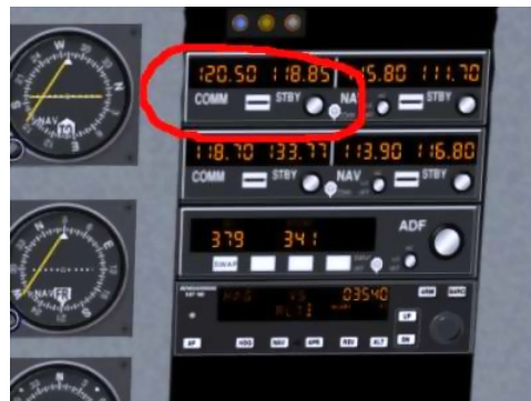
Figure 9.4: The C172 communications stack with COMM1 highlighted
