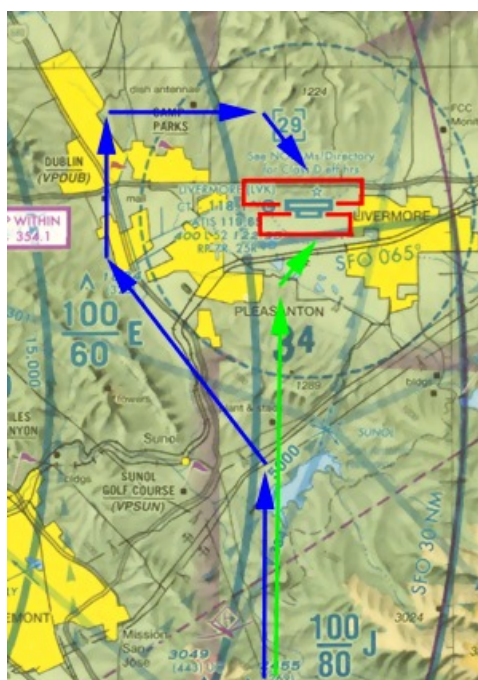
Figure 9.16: Sectional extract showing approaches to Livermore
