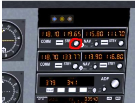
Figure 8.5: COMM1 adjustment knob
