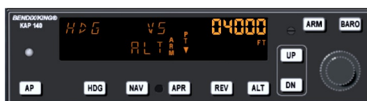
Figure 9.10: Autopilot with altitude armed
