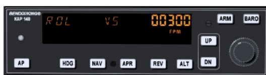
Figure 9.7: Autopilot after engaging
