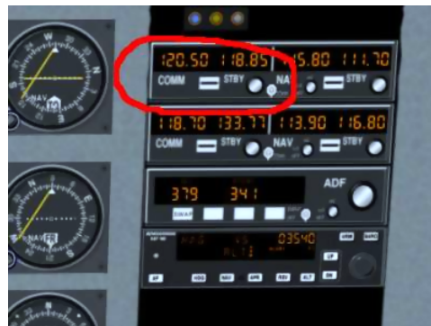
Figure 7.4: The C172 communications stack with COMM1 highlighted
