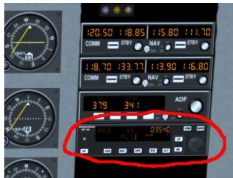
Figure 7.10: The C172 Autopilot
