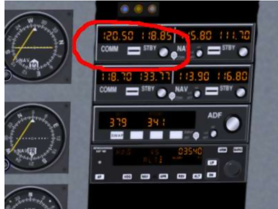
FIGURE 9.4 – The C172 communications stack with COMM1 highlighted
