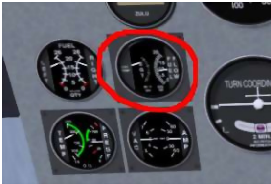
FIGURE 9.14 – Fuel Flow and EGT gauges
