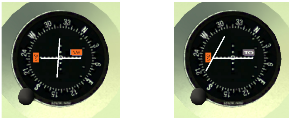
FIGURE 10.5 – VOR1, before and after tuning
