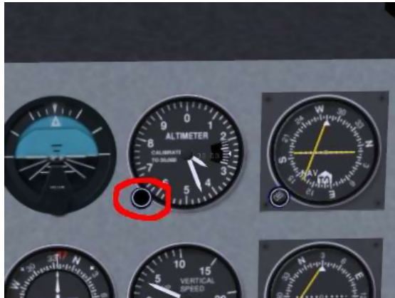
FIGURE 9.7 – Altimeter calibration knob
