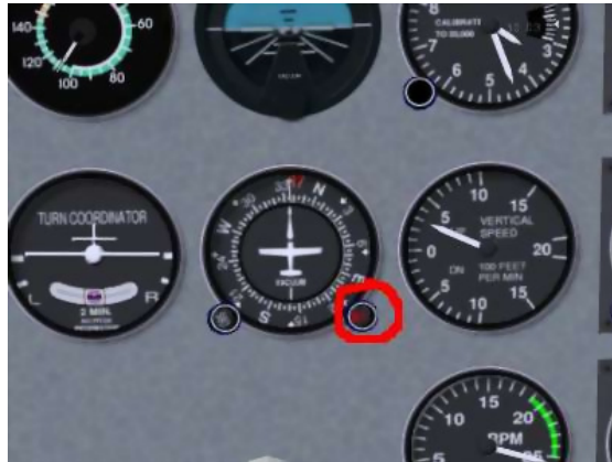
FIGURE 9.8 – Heading adjust knob
