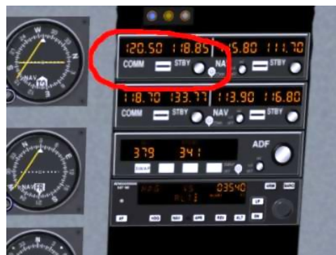
Figure 8.4: The C172 communications stack with COMM1 highlighted
