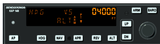
Figure 9.10: Autopilot with altitude armed
