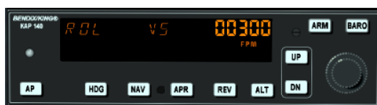
Figure 9.7: Autopilot after engaging
