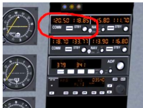
FIGURE 9.4 – The C172 communications stack with COMM1 highlighted
