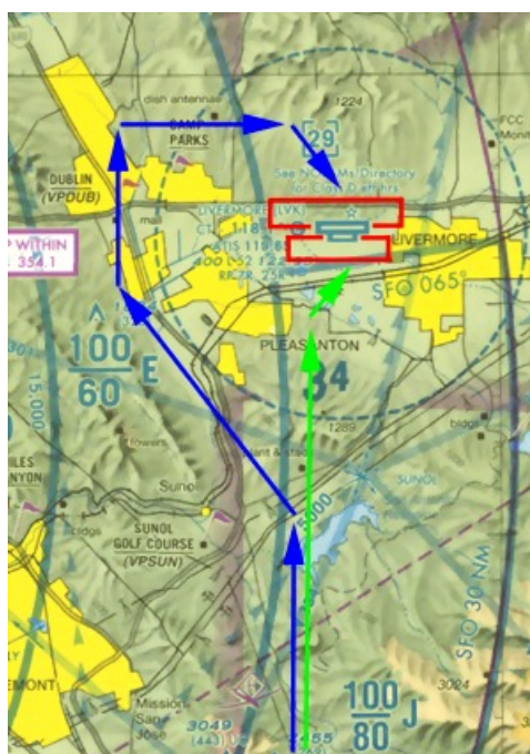
Figure 9.16: Sectional extract showing approaches to Livermore
