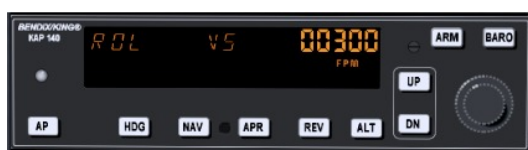
FIGURE 10.6 – Autopilot after engaging
