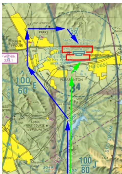
Figure 9.16: Sectional extract showing approaches to Livermore
