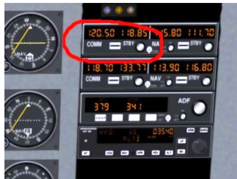
Figure 9.4: The C172 communications stack with COMM1 highlighted
