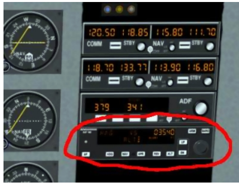
Figure 8.10: The C172 Autopilot
