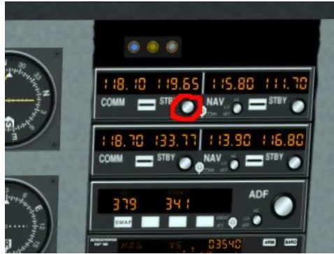
Figure 8.5: COMM1 adjustment knob
