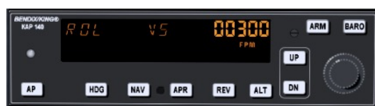
FIGURE 10.6 – Autopilot after engaging
