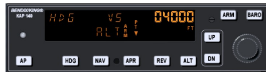
FIGURE 10.9 – Autopilot with altitude armed
