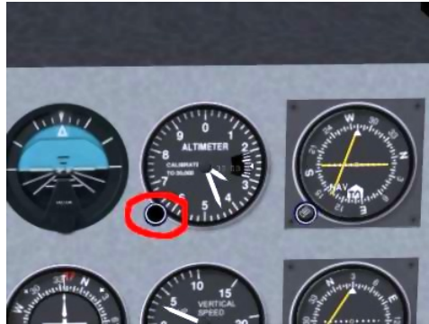
Figure 9.7: Altimeter calibration knob
