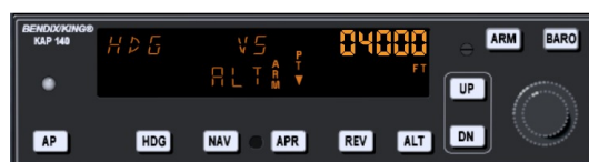
Figure 10.9: Autopilot with altitude armed
