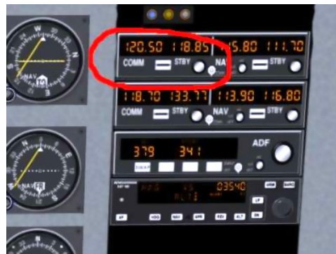
Figure 9.4: The C172 communications stack with COMM1 highlighted
