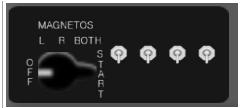
Fig. 4: The ignition switch.
