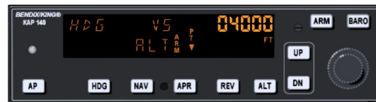
Figure 10.9: Autopilot with altitude armed
