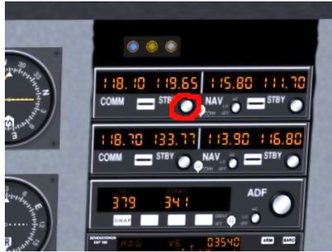
Figure 9.5: COMM1 adjustment knob
