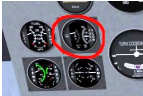
Figure 9.14: Fuel Flow and EGT gauges
