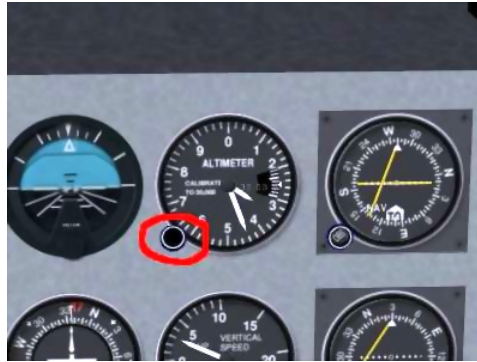
Figure 9.7: Altimeter calibration knob
