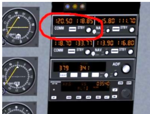
Figure 9.4: The C172 communications stack with COMM1 highlighted
