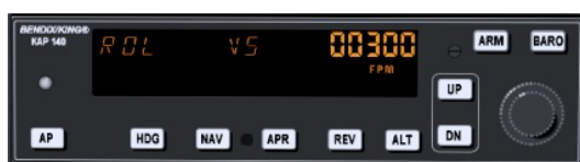
Figure 10.6: Autopilot after engaging
