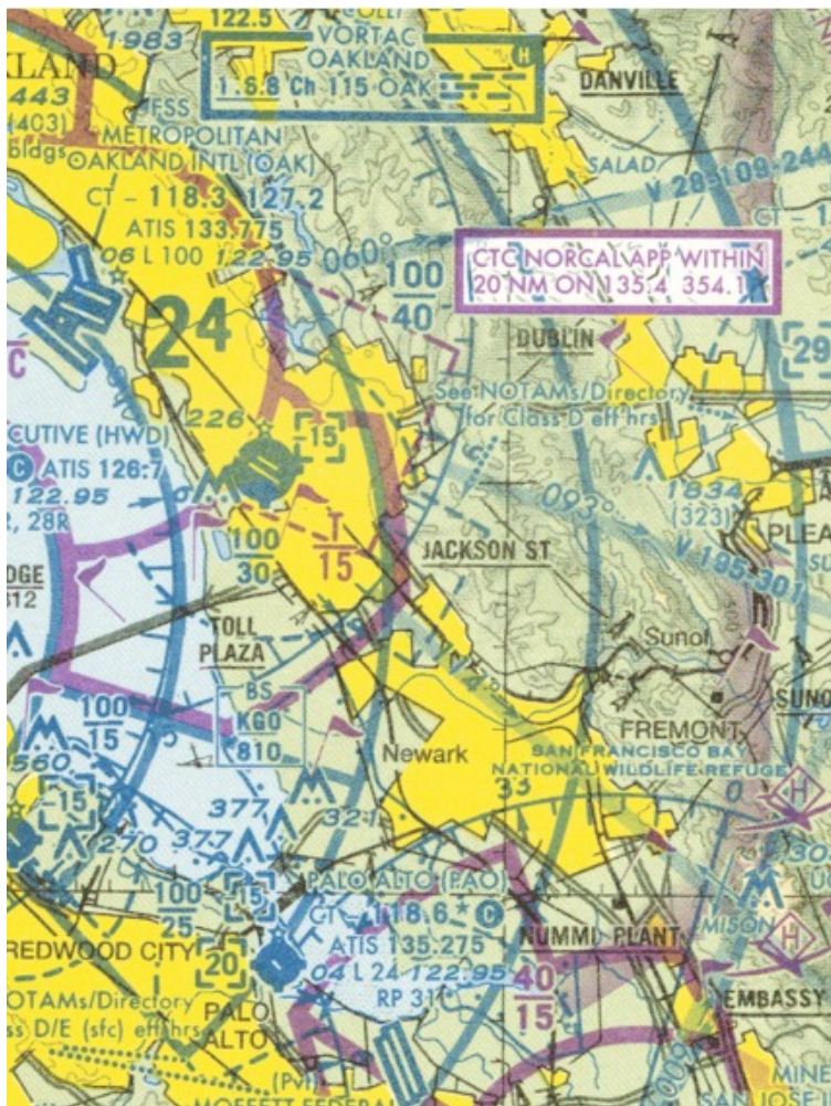
Figure 10.8: Oakland VOR and 114 radial to MISON intersection
