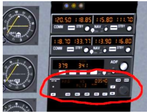
Figure 9.10: The C172 Autopilot
