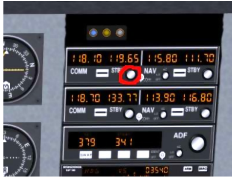
Figure 9.5: COMM1 adjustment knob
