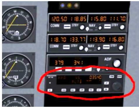
Figure 9.10: The C172 Autopilot
