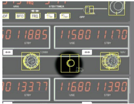
Figure 9.6: Ident volume knob and hot-spots
