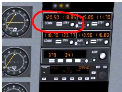
Figure 8.4: The C172 communications stack with COMM1 highlighted
