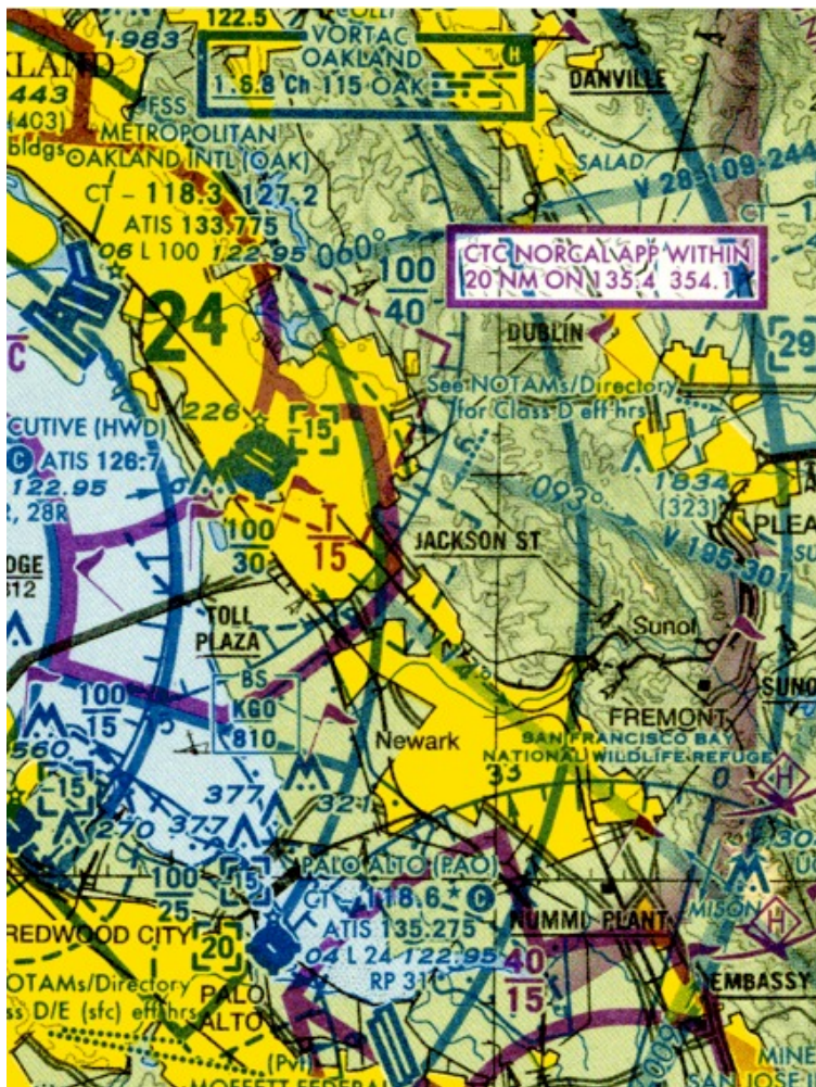
Figure 9.9: Oakland VOR and 114 radial to MISON intersection
