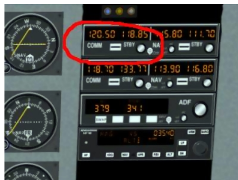
Figure 8.4: The C172 communications stack with COMM1 highlighted
