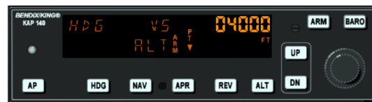
Figure 9.10: Autopilot with altitude armed
