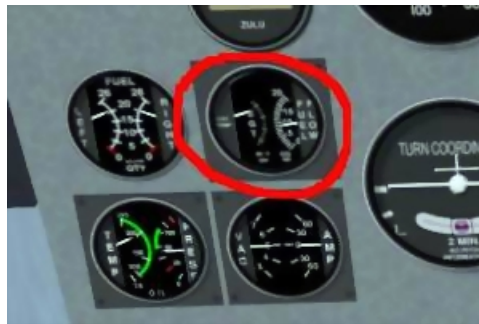
Figure 8.14: Fuel Flow and EGT gauges
