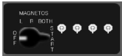
Figure 4.1: The ignition switch.
