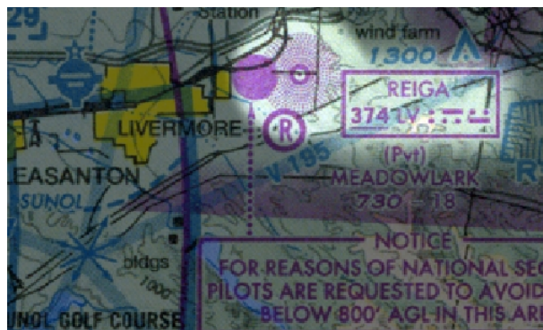
Figure 9.13: REIGA nondirectional beacon
