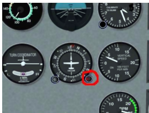
Figure 8.8: Heading adjust knob
