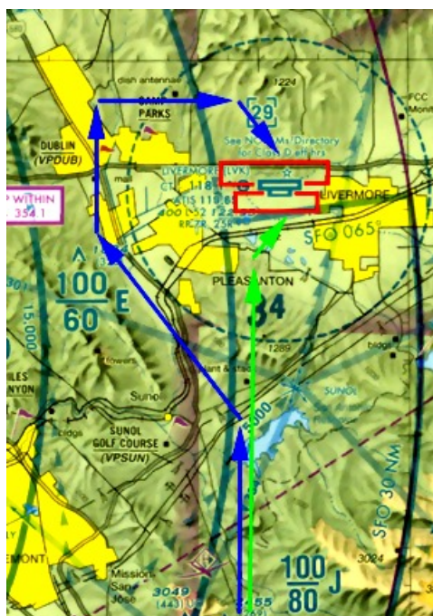
Figure 8.16: Sectional extract showing approaches to Livermore
