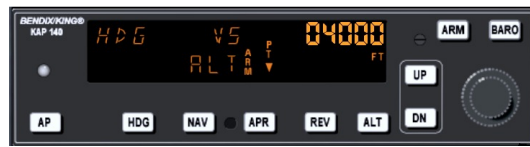
Figure 9.10: Autopilot with altitude armed
