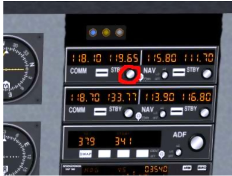
Figure 8.5: COMM1 adjustment knob
