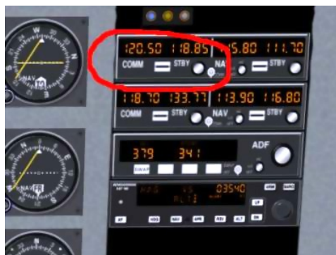
Figure 8.4: The C172 communications stack with COMM1 highlighted
