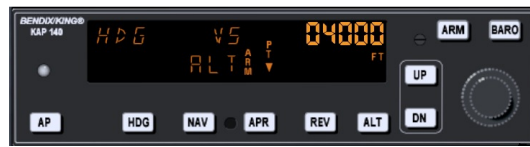
FIGURE 10.9 – Autopilot with altitude armed
