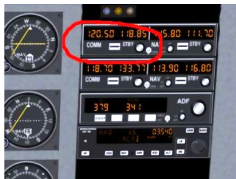
FIGURE 9.4 – The C172 communications stack with COMM1 highlighted
