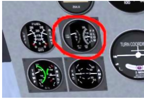
Figure 9.14: Fuel Flow and EGT gauges
