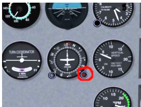
Figure 9.8: Heading adjust knob
